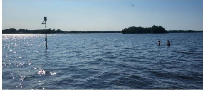
Figure 3-7 WISP station, constantly monitoring water quality on Paterswoldsemeer 56
